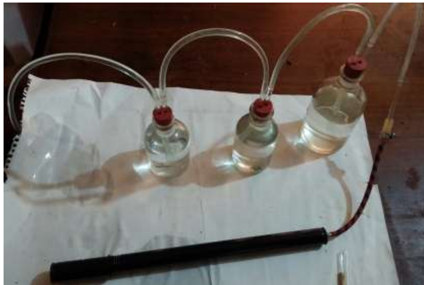
Plate 1. Photograph of assembled pump sampler for shallow water bodies.
